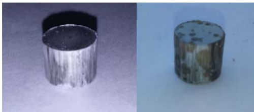
Fig. 2: Sample before and after sintering
